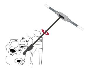
The size of the tap bits and the shoulder of their holder prevent any risk of tapping too far into the cylinder head without prior measurement
