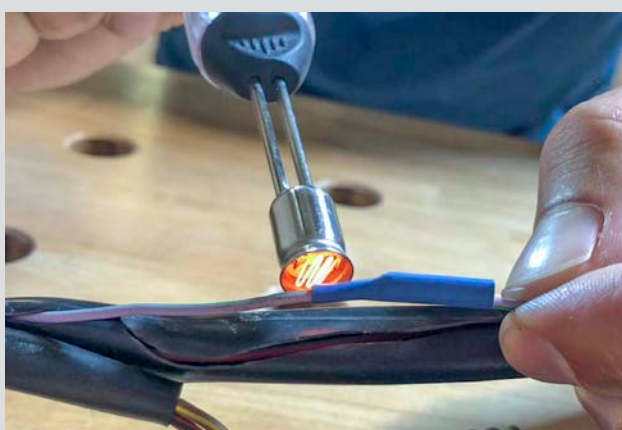
TIP FOR HEAT-SHRINK SHEATHS
