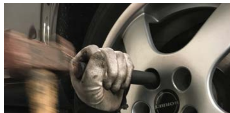
HAMMER EXTRACTOR INTO LUG
